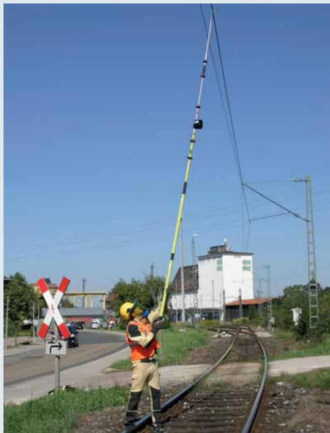
PHE voltage detector with visual indicator used on an overhead contact line of German Railways (DB)
