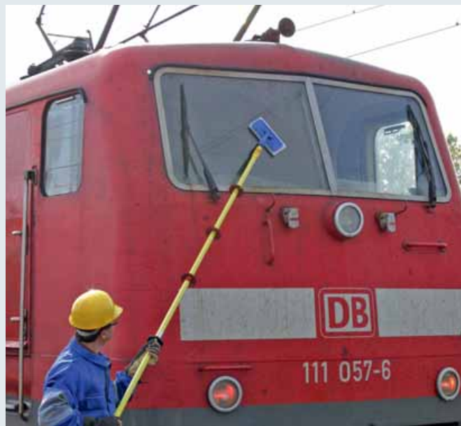
Insulating stick kit used for cleaning the windscreen of an electric locomotive
