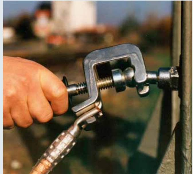
Universal earth clamp with handle connected to a fixed ball point
