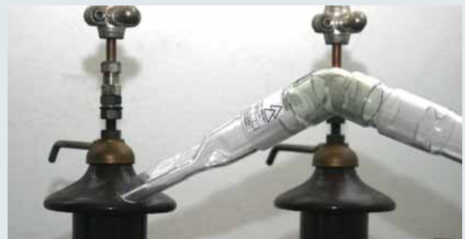
Cleaning an insulator with a flat cleaning head and 135° angled intake tube
