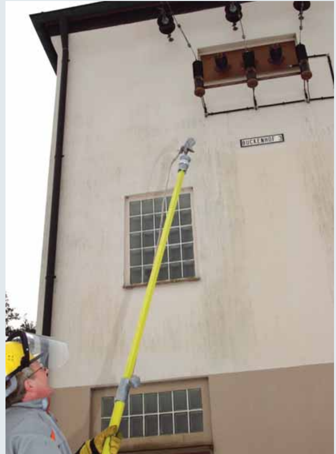
Telescopic earthing stick with aluminium cone coupling and phase screw clamp
